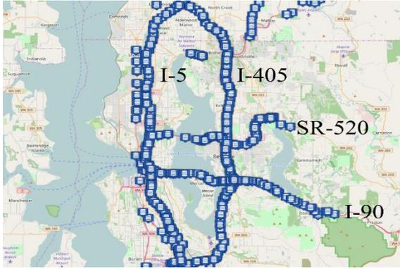
**Figure 5 Loop detector stations on the freeway network in Seattle area**
